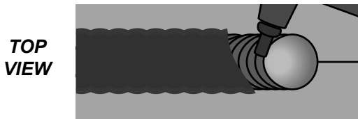
PARTIALLY CHIPPED AWAY TO SHOW WELD
